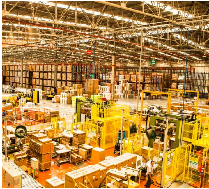
Translucent roof in Rio Claro Plant, Brazil
