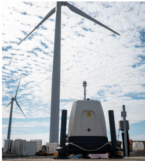
Our LiDAR units collect data about the wind. They transmit this data as 0s and 1s which our computers convert so that we can perform our wind analysis!
