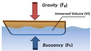
Buoyant Force = Density of Fluid \* 9.8  $\frac{m}{s^2}$  \* Displaced Volume of Fluid
