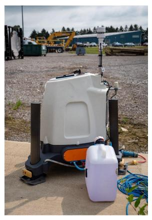
A close-up of a One Energy LiDAR near our office. The unit comes with a windshield wiper and washer fluid to keep the laser transmitting cleanly.
