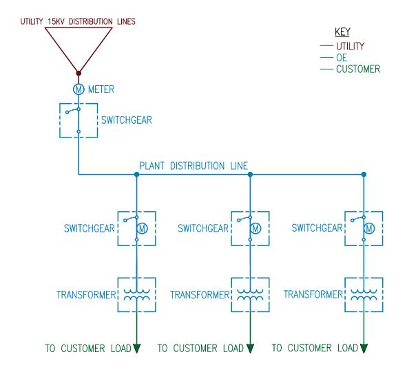
ONE-LINE DIAGRAM DEPICTING ONE POWER'S MANAGED HIGH VOLTAGE SERVICE AND HOW IT INTERCONNECTS WITH THE CUSTOMER'S FACILITY
